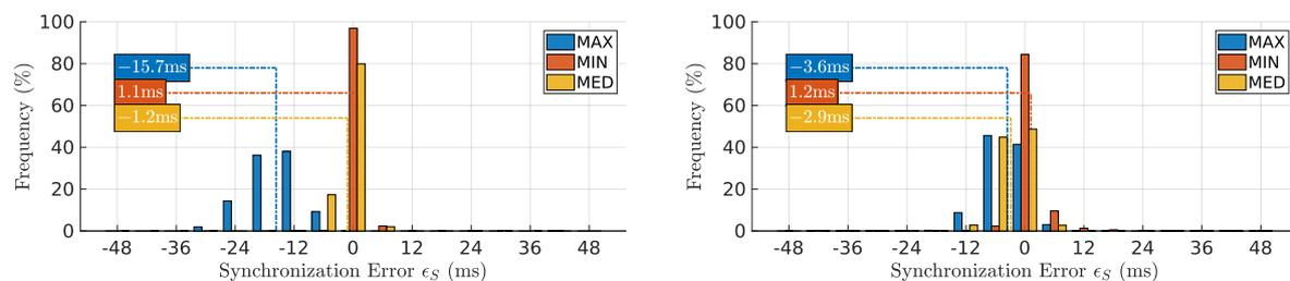
**Figure 8.** Distribution of synchronization error  $\epsilon_S$  on the first and second relays, left and right respectively. **MIN** shows the smallest synchronization error with a light gap. **MED**, delay's Median.
