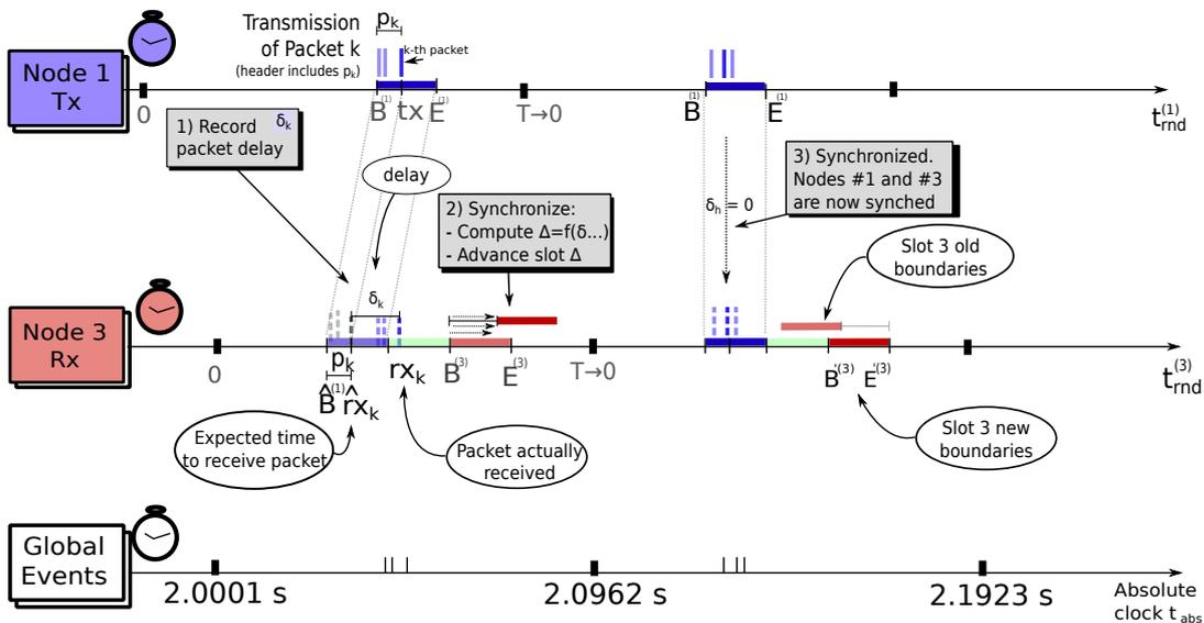
**Figure 7.** Shifting slots in the TDMA round to enforce synchronization. The upper timeline shows the local time frame of Node 1 as the transmitter, which was slightly advanced (blue slot). The middle timeline shows the local time frame of Node 3 as receiver, which senses Node 1 slot advancement and shifts its own slot (red slot), accordingly, maintaining synchronization. The lower timeline shows the global synchronization events, i.e., packets’ transmissions, on a virtual absolute time frame.
