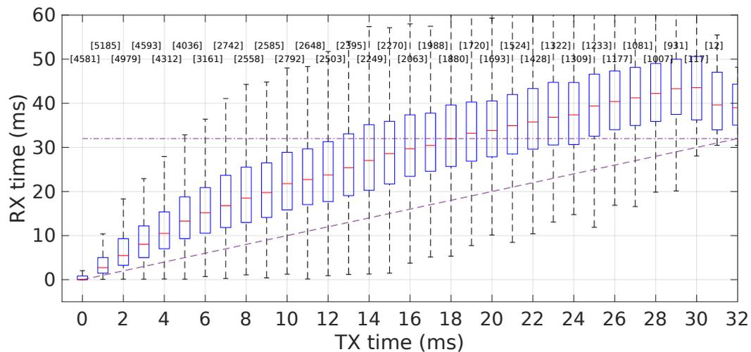
**Figure 14.** Packet spreading. Packets reception times ( $y$ -axis) as a function of the respective transmission times ( $x$ -axis) in the transmitter slot, at the application layer. Reception times grow visibly along the slot, due to packet accumulation in queues.
