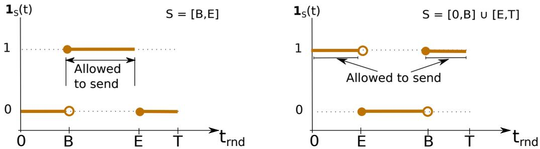
Figure 4. A TDMA transmission slot  $S$  is defined by its boundaries  $B$  and  $E$ . A node is allowed to transmit packets if current round-time  $t_{rnd}$  is within  $S$ , i.e., if  $1_S(t_{rnd}) = 1$ .
