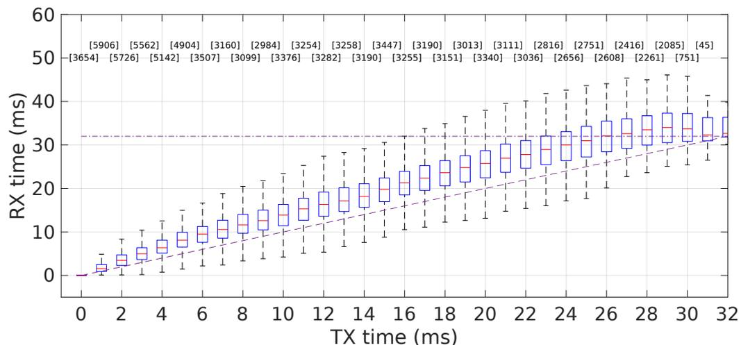
**Figure 15.** Packet spreading is strongly reduced upon deployment of a transmission control policy at the socket send queue level (maximum amount of unsent data allowed set to 100 B). This policy was used in the experiments reported in the Results Section.
