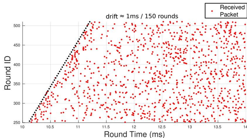
**Figure 13.** Nodes synchronized using NTP at the beginning of the mission, only. Per line, we can see the reception instants of packets sent by the source in the corresponding receiver slot at the first relay. The transmitter and receiver slots show a clear drift of, approximately, 1 ms every 150 rounds (drift 1:14,400).
