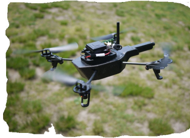
Figure 3.1: AR Drone 2.0 platform, a common COTS quadrotor, used for the experiments.
