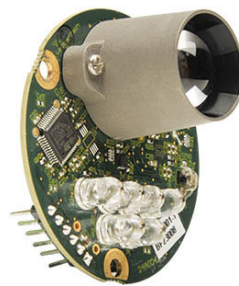
Figure 1.6: LeddarOne is a LIDAR sensor designed for small UAVs.
