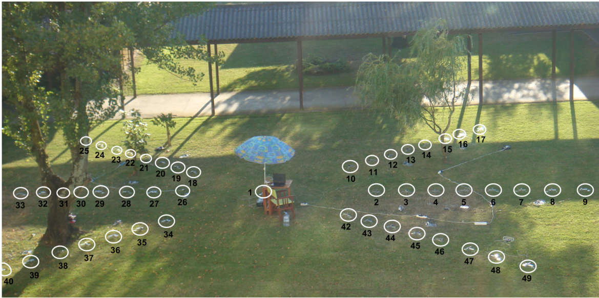
Figure 5.1: Nodes Distribution According the Circular Topology, in a Garden of ISEP
