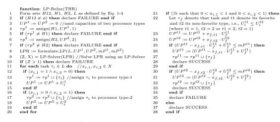
Figure 1: The LP-Relax(THR) algorithm for assigning tasks on to a two-type heterogeneous multiprocessor platform.
