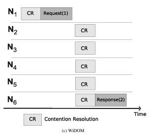
Figure 1. Illustrations: (a) (#Nodes -1) responses as a result of the MIN request of  $N_1$ , (b) Bit-wise arbitration, (c) Only one response is generated for the same request.
