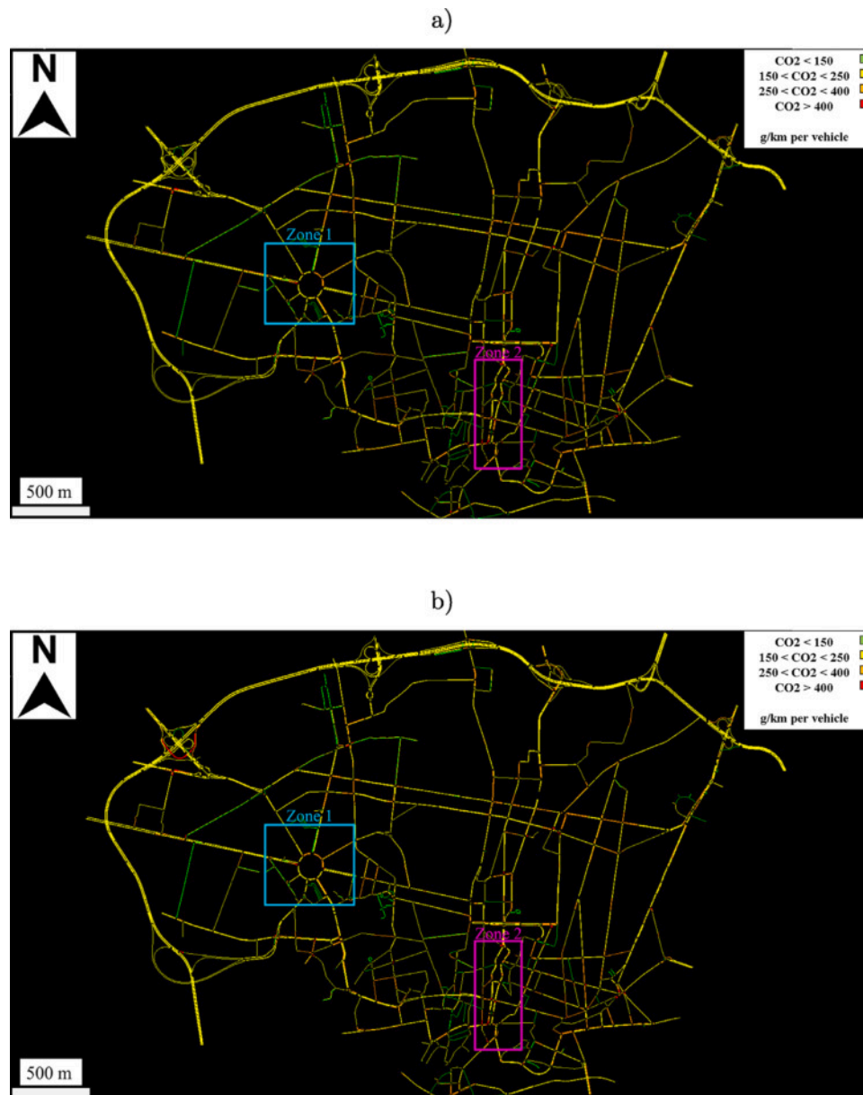
Fig. 8. Spatial distribution of CO 2 emissions locations per unit distance in the baseline scenarios: (a) 6–7 AM.; and (b) 8–9 AM.
