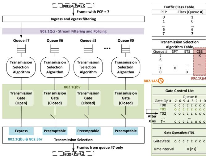
Fig. 4. TSN enhancements to the forwarding process of IEEE 802.1Q VLAN bridges
