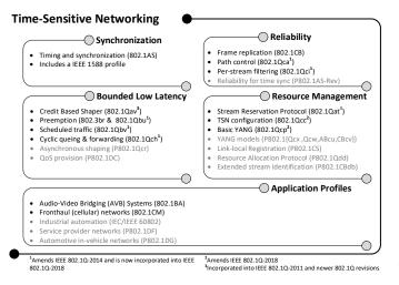
Fig. 3. Time-Sensitive Networking (TSN) set of standards/amendments [20]
