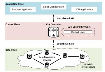
Fig. 1. Architecture of an SDN-enabled network
