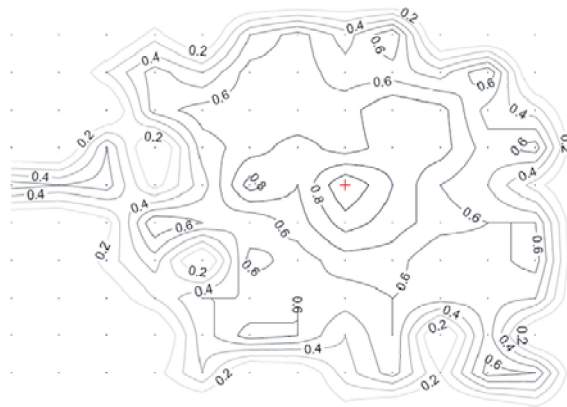
Fig. 4. Contour of PRR from a central node: anisotropy of link quality [Ganesan et al. 2002].
